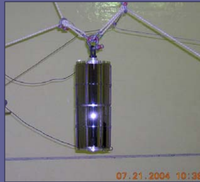
Prototype glass mirror acoustics tested at JPL facility
