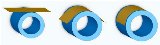
Mirror segment on a precisely figured mandrel
