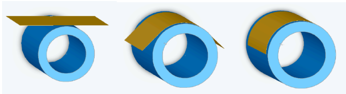
Mirror segment is produced by thermal forming of a thin glass sheet on a precisely figured mandrel
