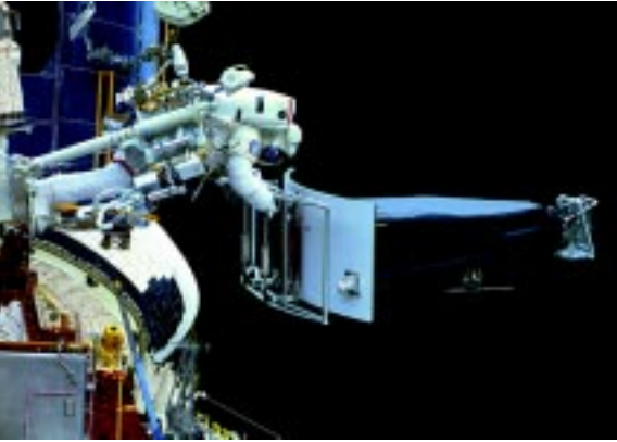
Wide-Field Planetary Camera being removed on-orbit during the first Servicing Mission.
