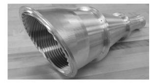
FIG. 3. Photograph of the 10 GHz horn.
