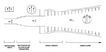
FIG. 1. Schematic of the horn system.
