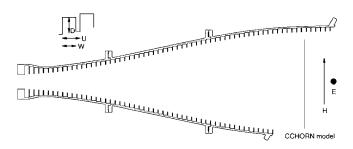
FIG. 2. Profile of the 10 GHz horn as designed, with a close-up showing dimensional parameters. The extent of the modeled unsliced horn is shown, as are the directions of the E and H planes as referred to in the article.
