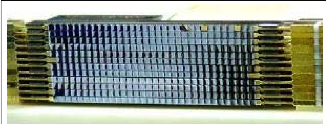
Figure 4-6. HAWC engineering prototype array for the SHARC II instrument. The array is a 12x32 (384 pixel) format
